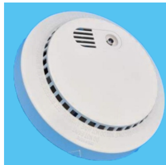
SMOKE DETECTOR Model DFS425 Operated voltage-9V Battery(include); Sensor:Optical sensor; Sensitivity-0.086DB/M to 0.140DB/M; Alarm sound: \geq 85dB(3M) ;
