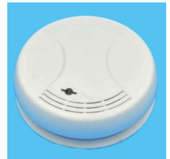
SMOKE DETECTOR Model DFS427 Operated voltage-9V Battery(include); Sensor:Optical sensor; Sensitivity-0.086DB/M to 0.140DB/M; Alarm sound: \geq 85dB(3M) ;
