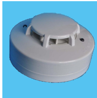
SMOKE DETECTOR Model DFS515 Operated volt-9VDC-35VDC; Sensor:Optical sensor; Sensitivity-0.15 dB/m( \pm 0.03 dB/m); Standby current: \leq 50\mu A (2 wires); Alarm current: \leq 50mA ;
