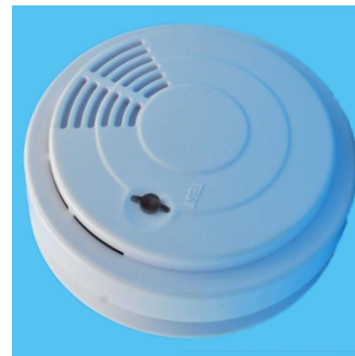
SMOKE DETECTOR Model DFS426 Operated voltage-9V Battery(include); Sensor:Optical sensor; Sensitivity-0.086DB/M to 0.140DB/M; Alarm sound: \geq 85dB(3M) ;
